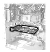
Seat the board securely into the slot.
